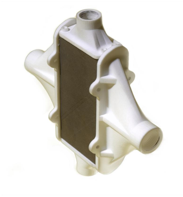
Figure 57: SLS test piece assembly mock-up
