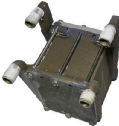
Figure 22: Water-to-water Ti64 heat exchanger [67]
