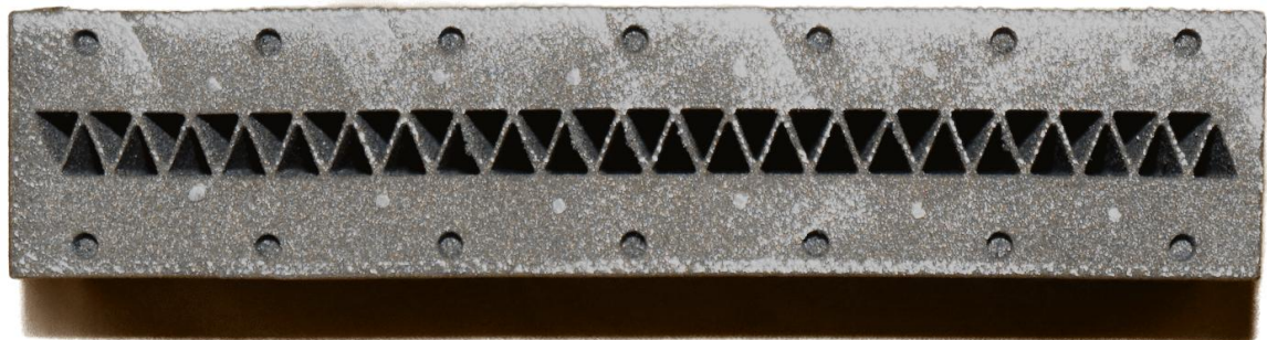
Figure 54: Test piece hot side channels
