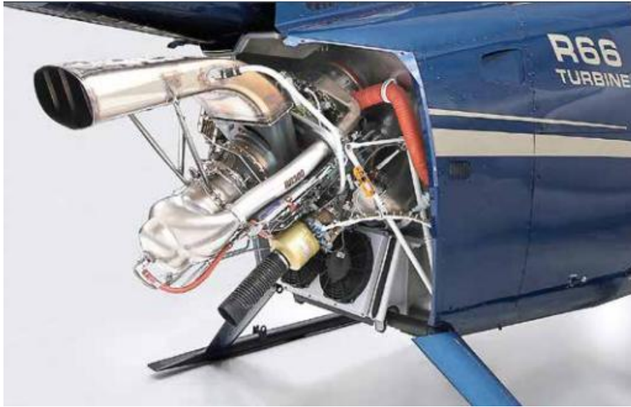
Figure 26: Robinson R66 turbine helicopter turboshaft engine [68]
