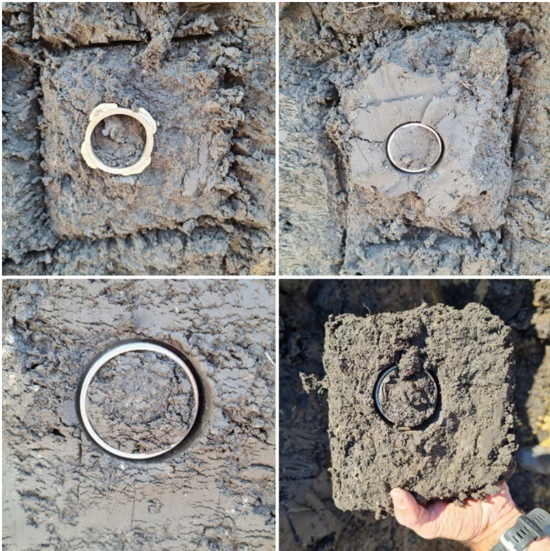
Figure 3-6: Sample collection for FC testing
