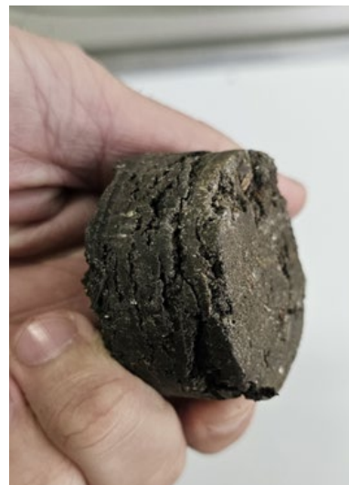
Figure 4-7: Sample shear during sample collection
