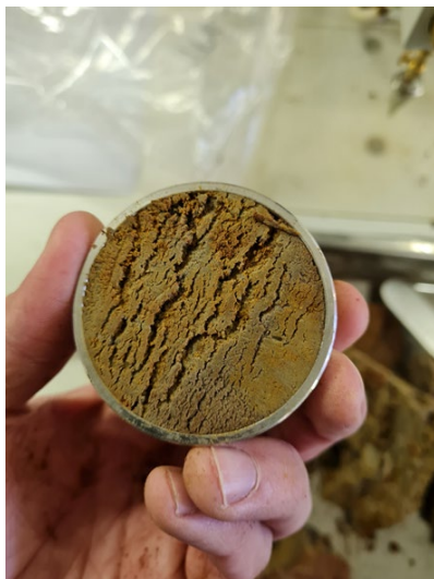
Figure 4-6: FC sample after cutting
