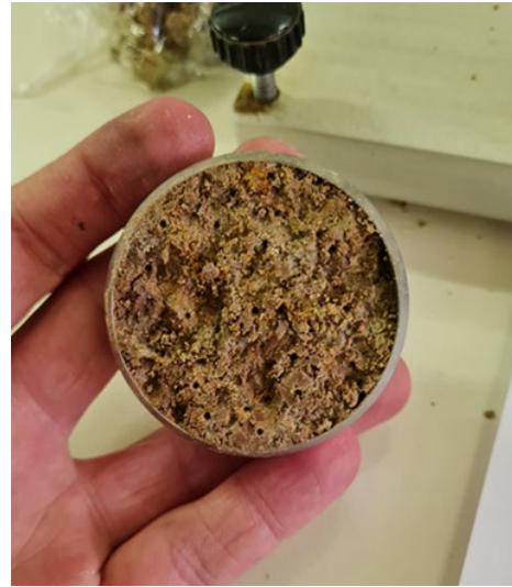
Figure 4-5: Disintegrating FC sample
