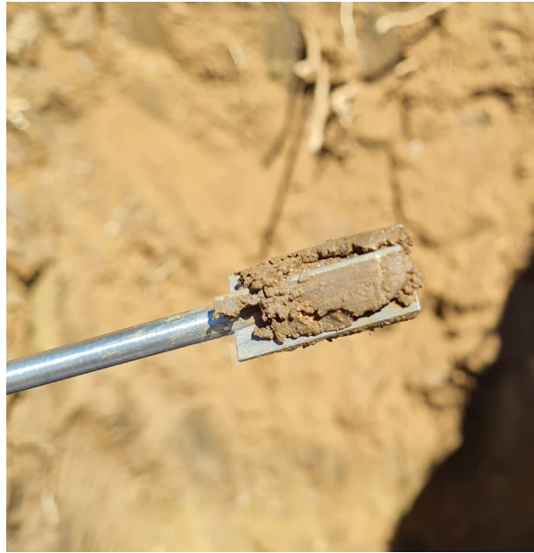
Figure 4-1: Vane blade after testing
