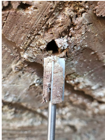
Figure 3-5: Vane shear after testing
