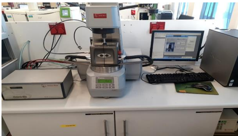
Figure 4.4 The equipment that was utilized to determine the dynamic rheological measurements
