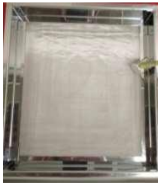
Figure 3.2: Manual sieve used to sieve Ti6Al4V(ELI) powder at CRPM
